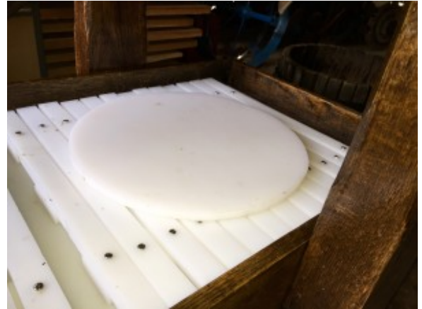
Base Plate for Tub Press
